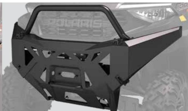
4.4 cm DIAMETER STEEL TUBE CONSTRUCTION
